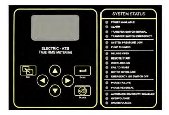
**Description**—Firetrol® FTA1800 Autotransformer Starting Fire Pump Controllers use an autotransformer to supply reduced voltage when starting the motor. The control-ler is of the closed circuit type where the motor circuit remains closed during the transition from start to run resulting in minimum line disturbance.
